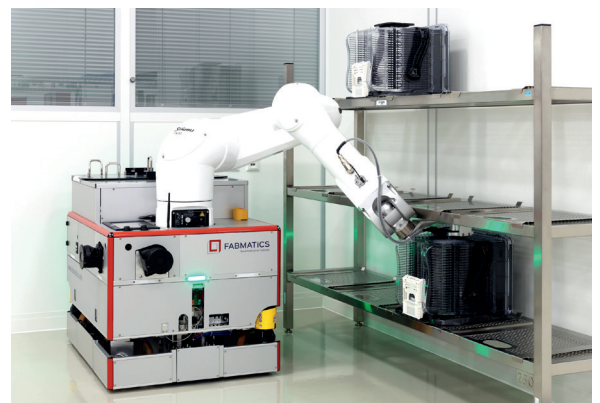
HERO Fab 300 loading 3 rack levels
