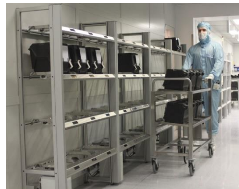
Operator with RFID trolley at RFID racks
